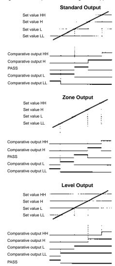
Note: The following setting conditions must be satisfied, otherwise no zone output will turn ON correctly.
